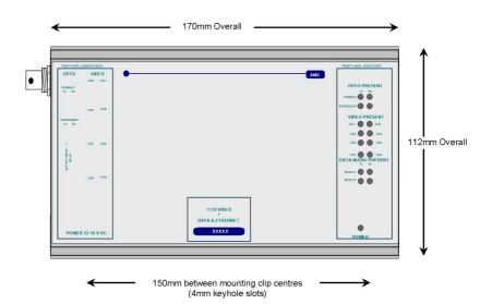
The **AMG4713E** is a standalone single channel video transmit unit designed to transmit 1 video signal and transmit and receive 1 data signal plus full duplex 100BaseT Ethernet connectivity over two singlemode fibres.
